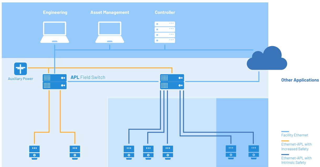
**Figure 4:** Example topology for a compact star installation
