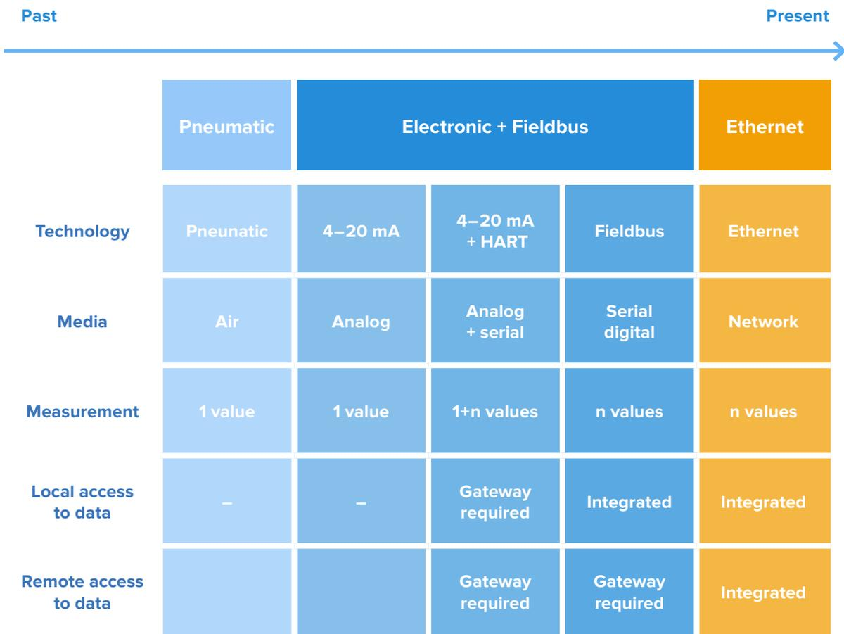
**Figure 1:** Technologies for the field of process automation
