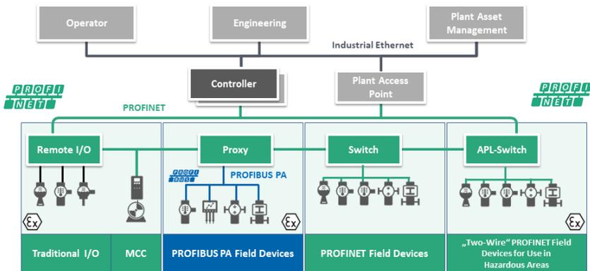
Fig. 3: PROFINET and PROFIBUS PA, and in the future with APL
