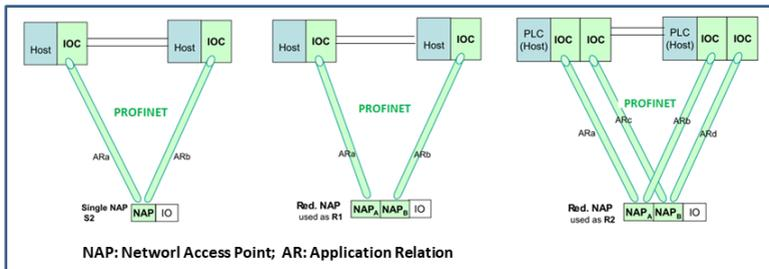
Fig. 13: System redundancy
