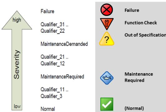
Fig. 8: Assignment of the PROFINET device diagnostics to NAMUR NE 107 requirements
