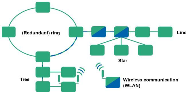
Fig. 4: Flexible network configuration of PROFINET
