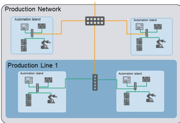
Fig. 10: Segmentation of the network
