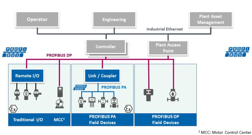
Fig. 2: Communication structure of a plant with PROFIBUS DP and PROFIBUS PA
