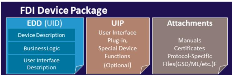
Fig. 17: The FDI technology building blocks
