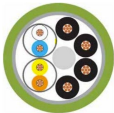
Figure 20: Cable example cross section 2-pair hybrid
