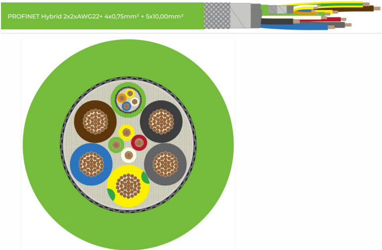
Figure 21: Cable example cross section 2-pair hybrid
