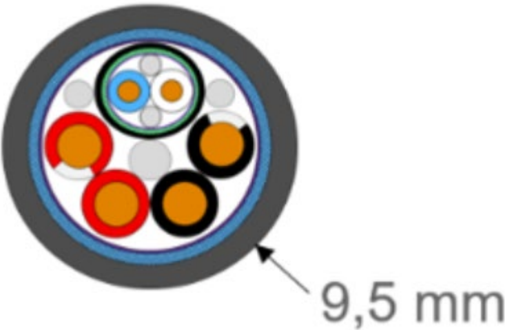
Figure 14: Cable example cross section 1-pair hybrid
