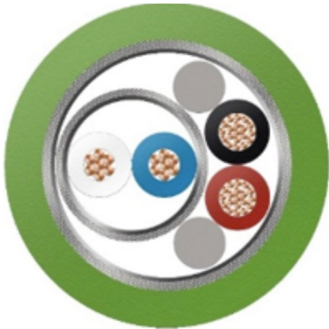
Figure 12: Cable example cross section 1-pair hybrid
