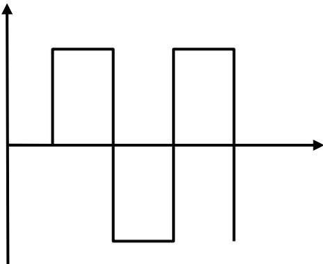
Overlaid signal (original signal + reflection) for too little terminating resistance
