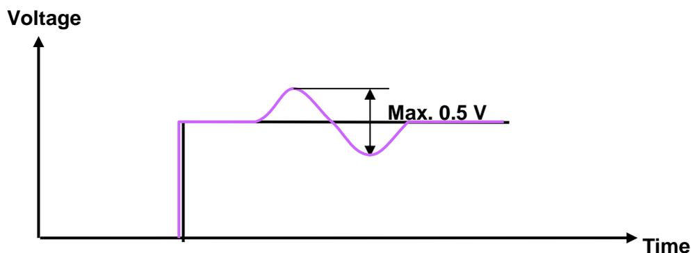
Figure 5-6: Signal waveform for non-connected PROFIBUS stations
