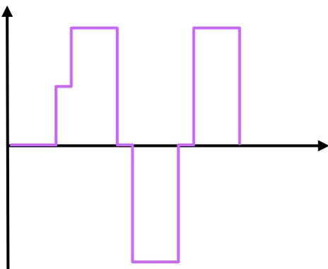
**Figure 5-8: Missing terminator**
