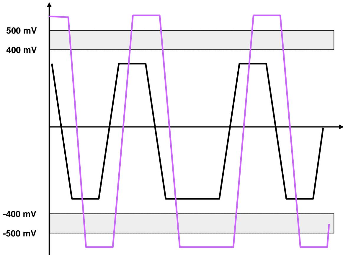
Figure 5-10: PROFIBUS MBP (PA) with defective bus terminator
