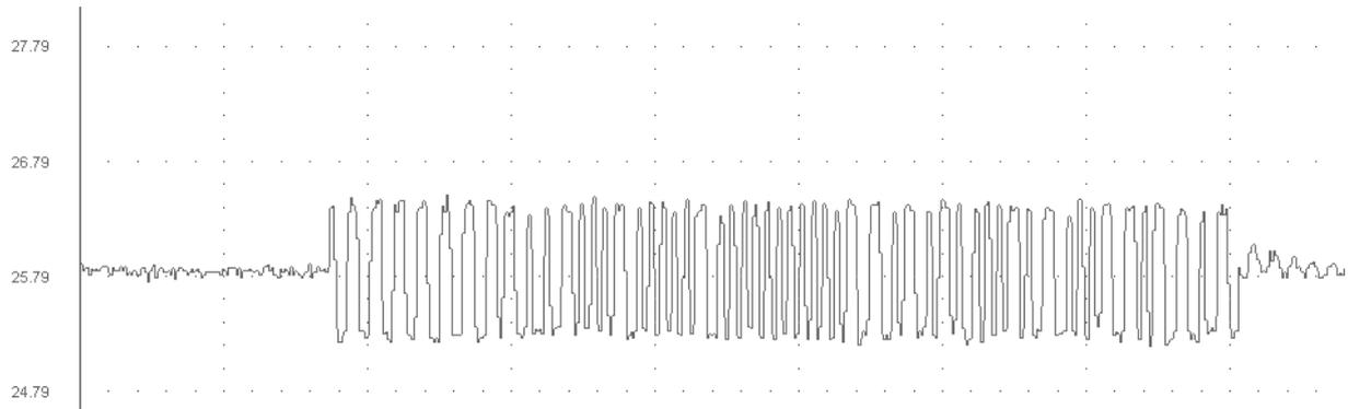
**Figure 5-11: Measurement PROFIBUS MBP (PA) (1 telegram)**
