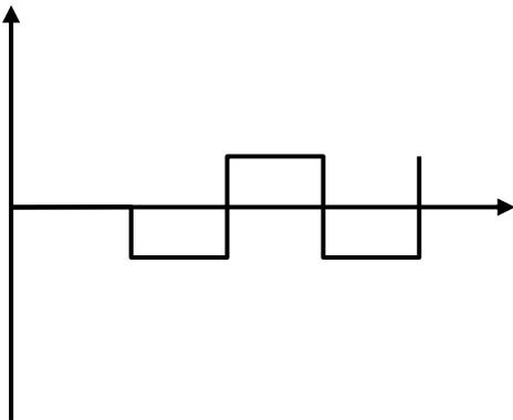
Overlaid signal (original signal + reflection) for too much switched-on terminator resistance
