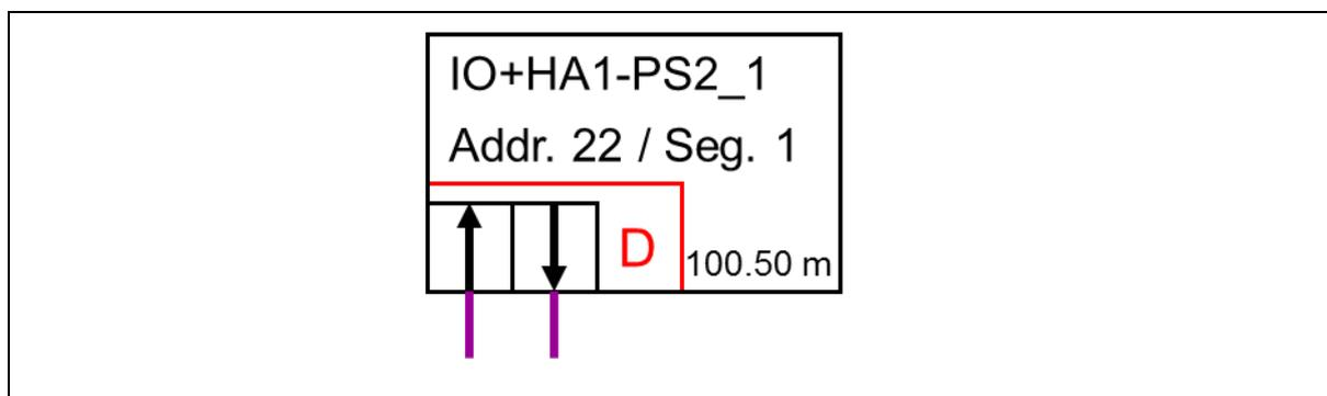
Figure 6-8: Example of PROFIBUS forwards documentation, diagnostic port example
