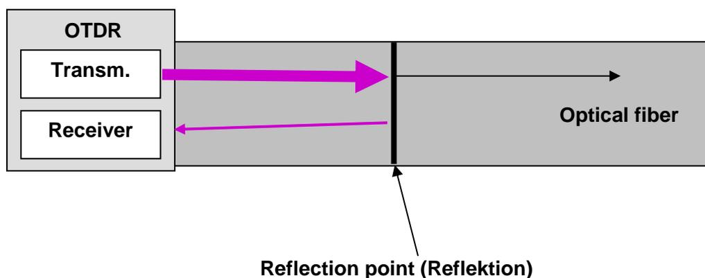
Figure 2-2: OTDR measurement principle
