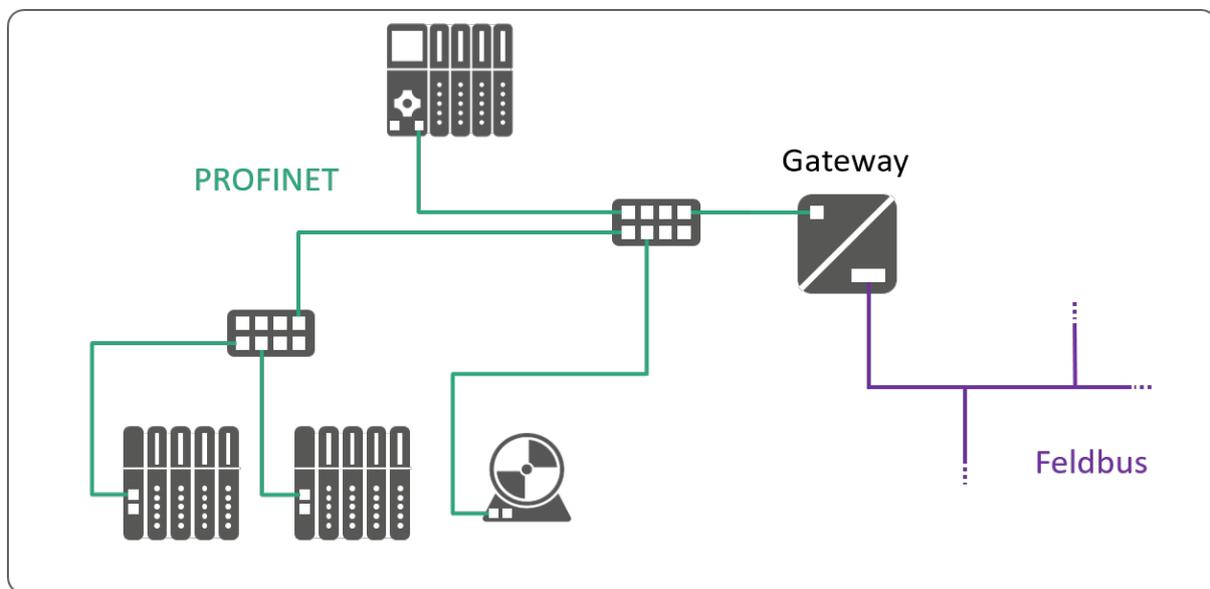
Figure 3-13: Use of a gateway to connect a fieldbus
