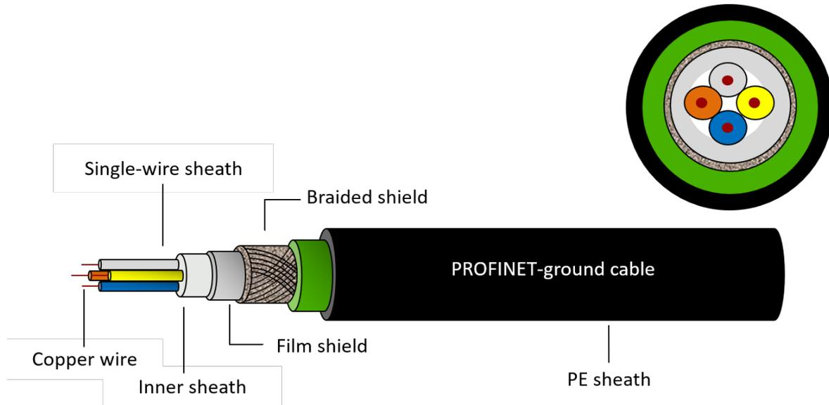
Figure 10-3: PROFINET ground cable
