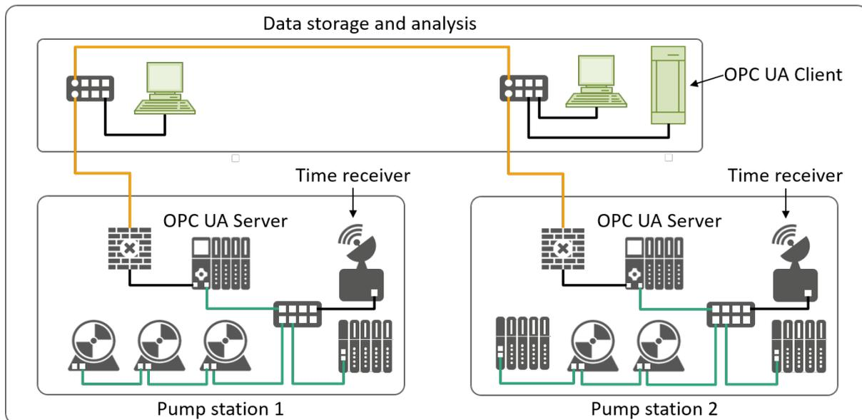
Figure 6-6: Plant example of data analysis and Sequence of Events
