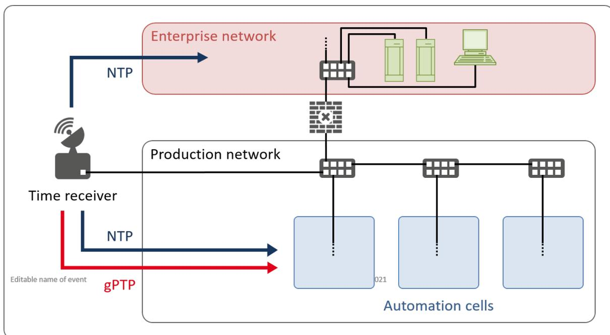
**Figure 4-1: Possible architecture for the distribution of time information**
