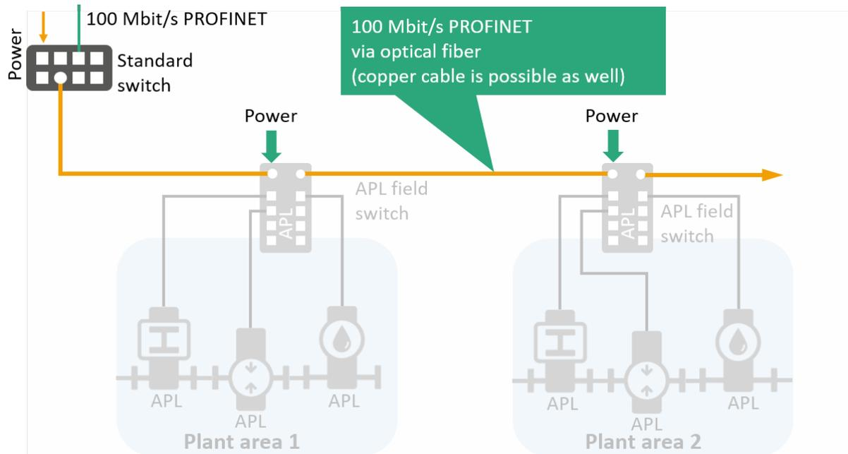
**Figure 5-2: Field switches with Industrial Ethernet connection**
