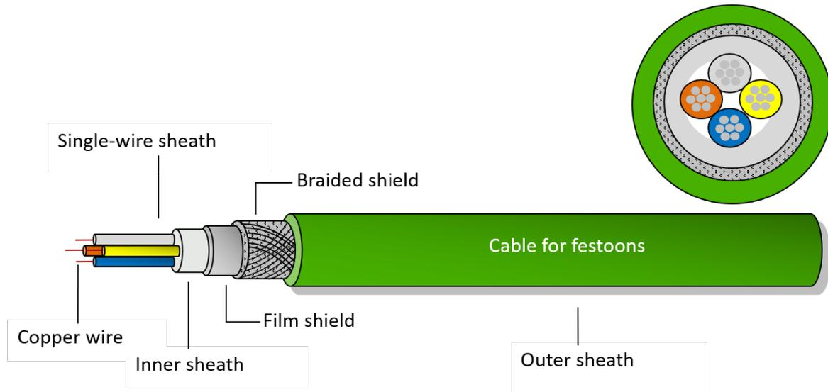
Figure 10-5: Cables for festoons
