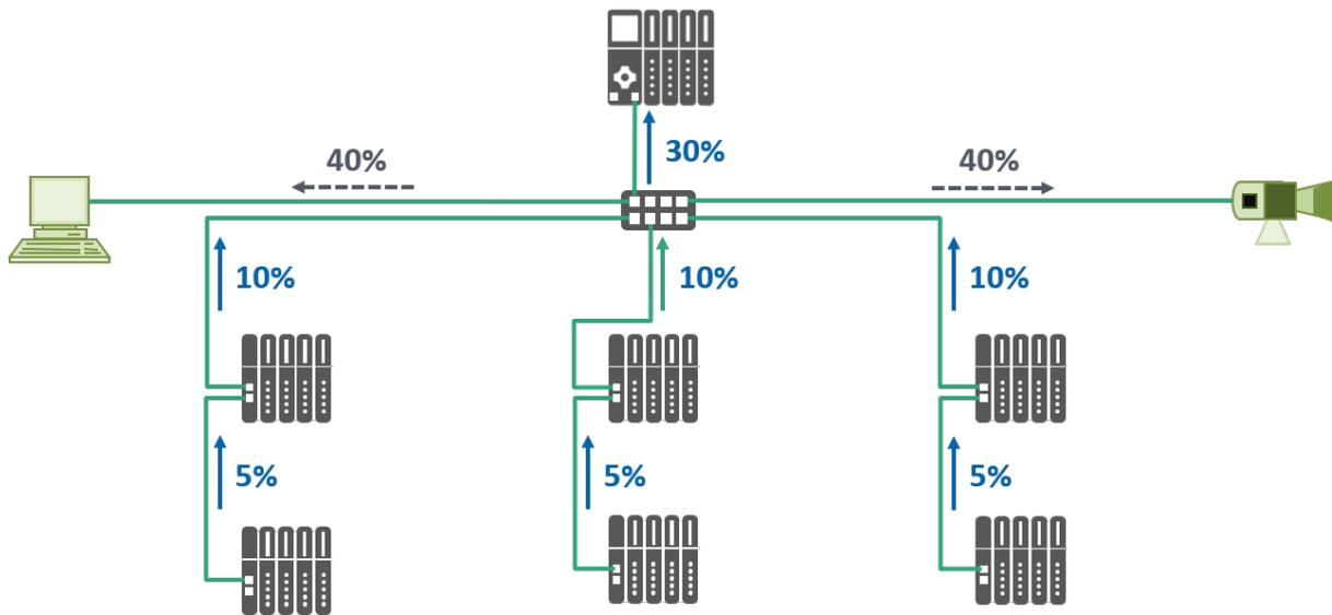
**Figure 7-20: Optimized topology with reduced network load**
