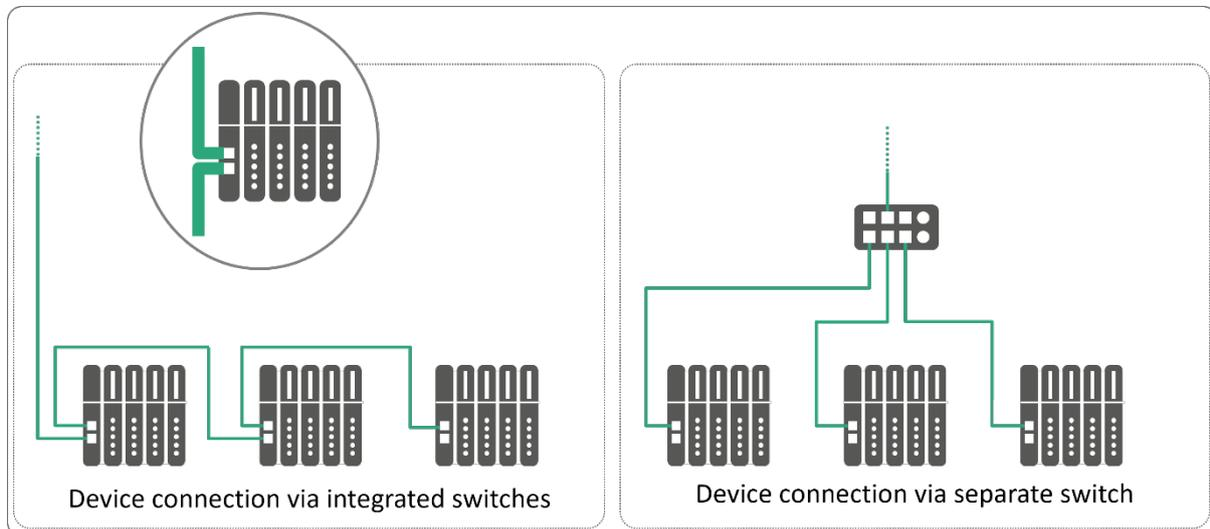
**Figure 3-2: Difference integrated switch and separate switch**
