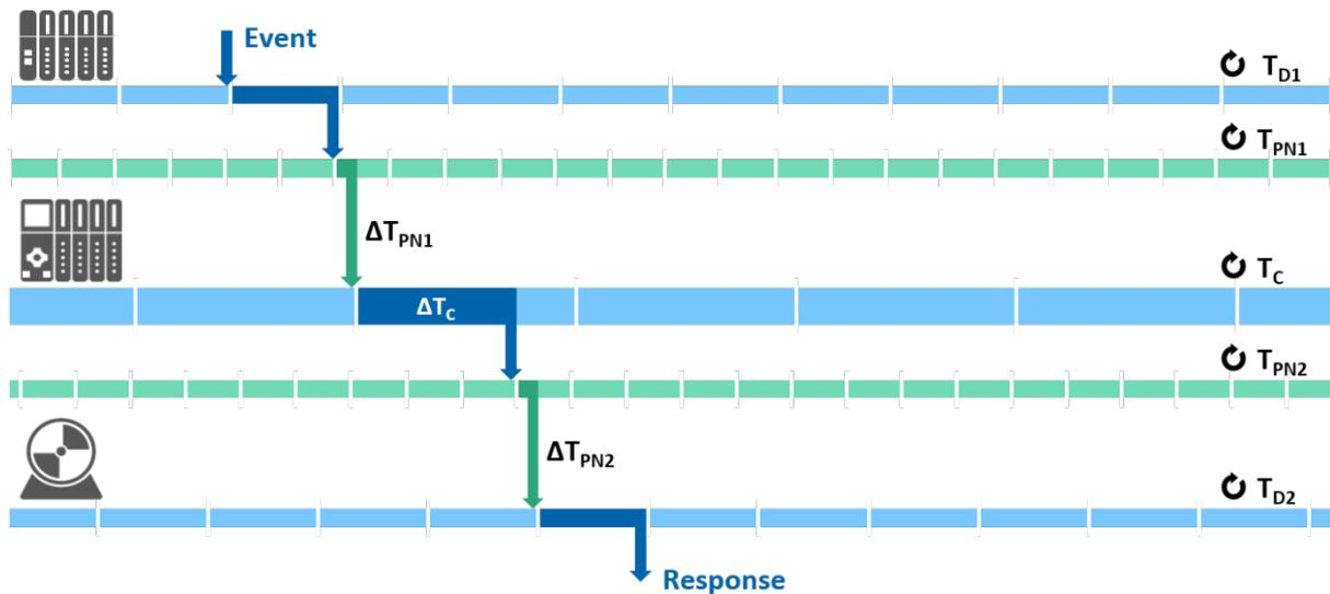
Figure 7-7: Examples of cycles in the processing chain, shortest response time
