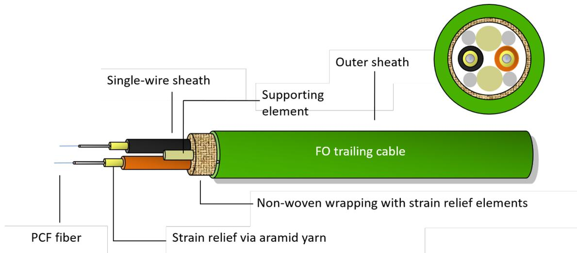
Figure 10-8: PROFINET FO trailing cable
