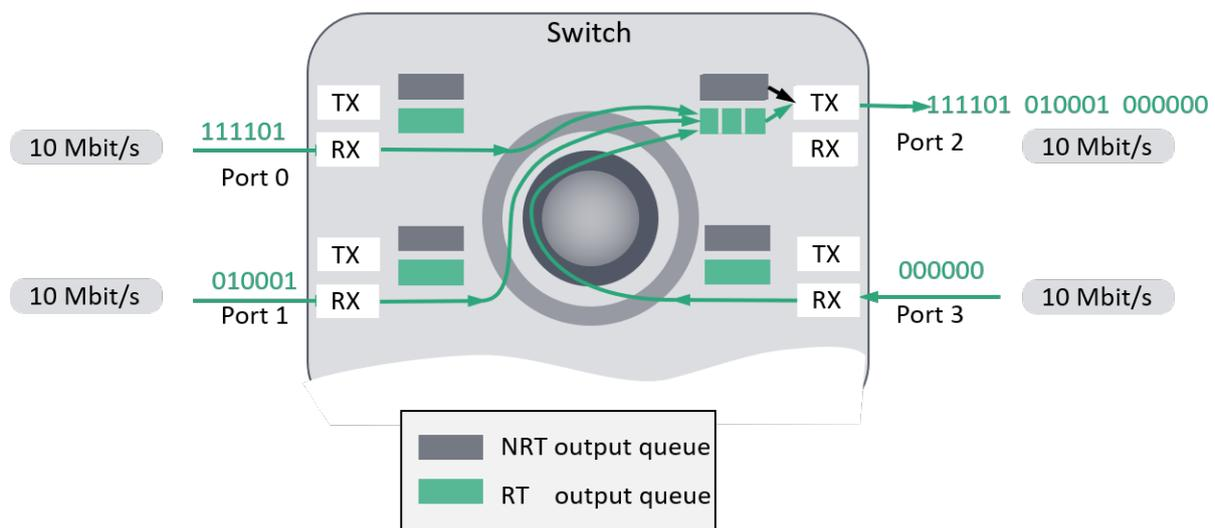
**Figure 7-23: Congestion loss due to input/output unbalance port wise**
