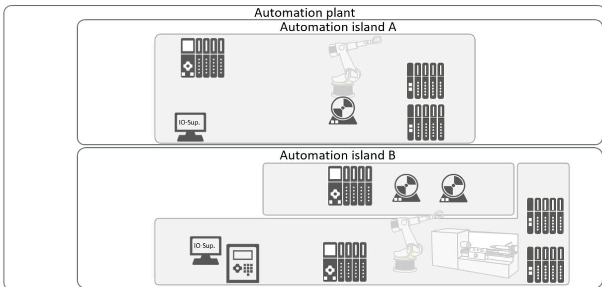
**Figure 2-2: plant example with spatial and functional clustering**
