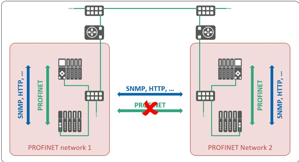
**Figure 3-3:Using a router in PROFINET networks**
