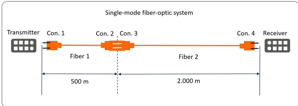
**Figure 10-22: Representation of attenuation balance for single-mode optical fiber links**
