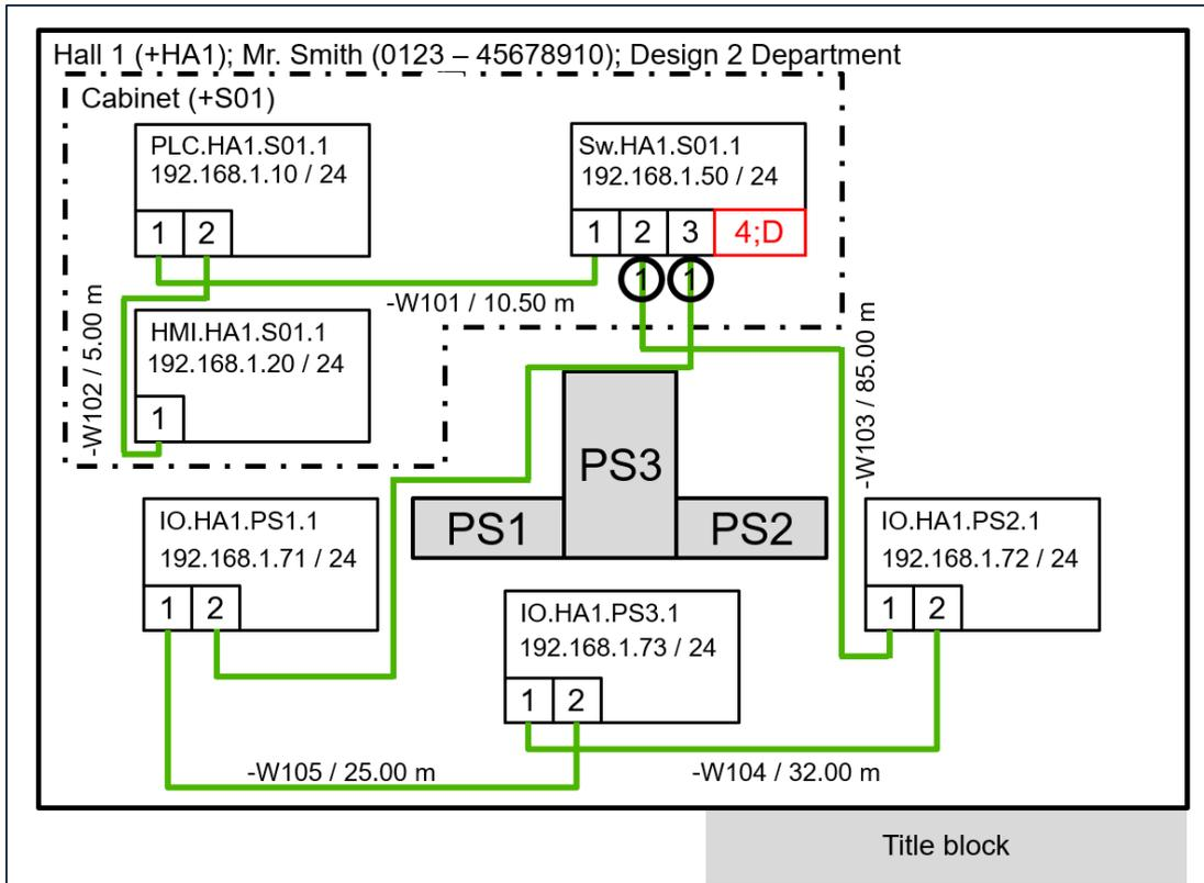
Figure 10-29: Example of PROFINET forwards documentation, ring topology
