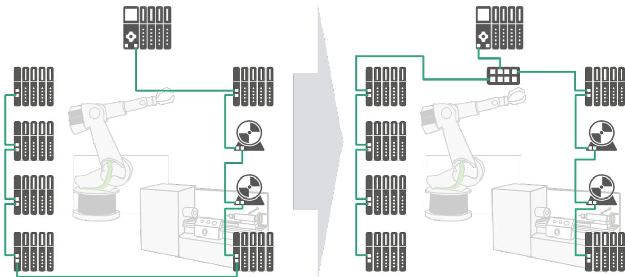
**Figure 7-13: Example of reduced line depth**
