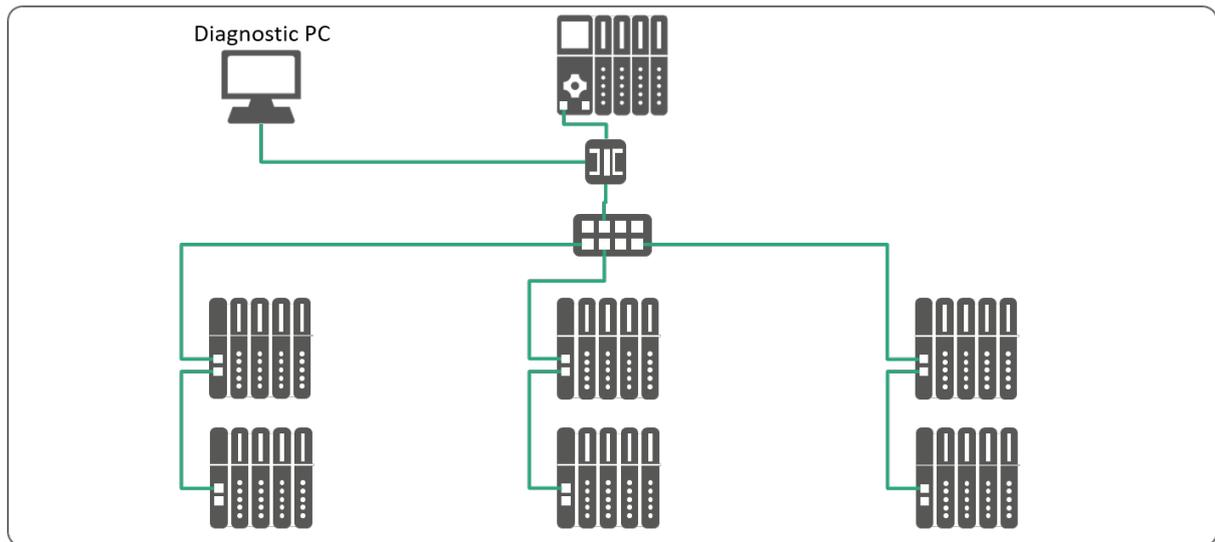
**Figure 4-8: Reading data streams via TAP**
