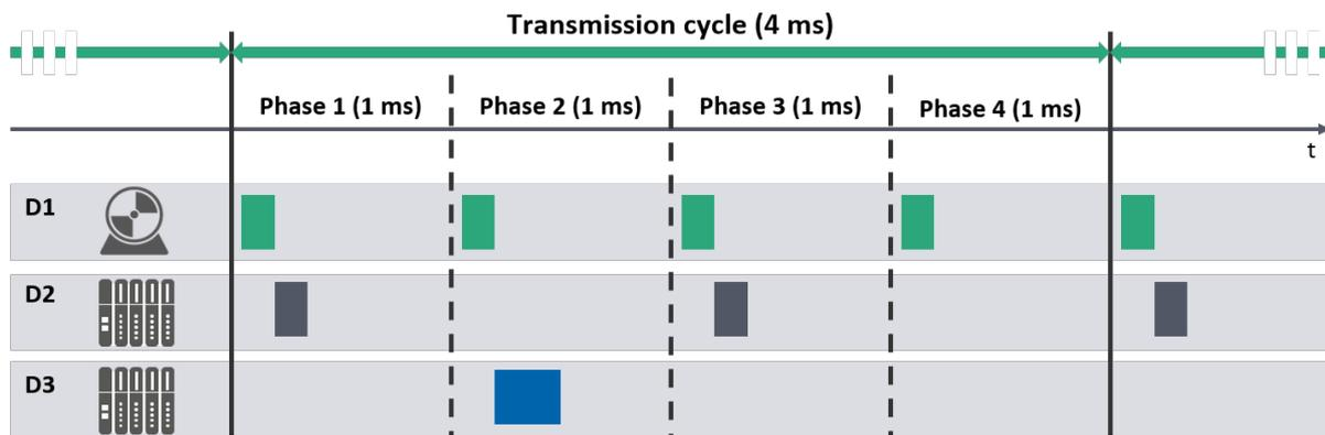
Figure 7-2: PROFINET transmission cycle
