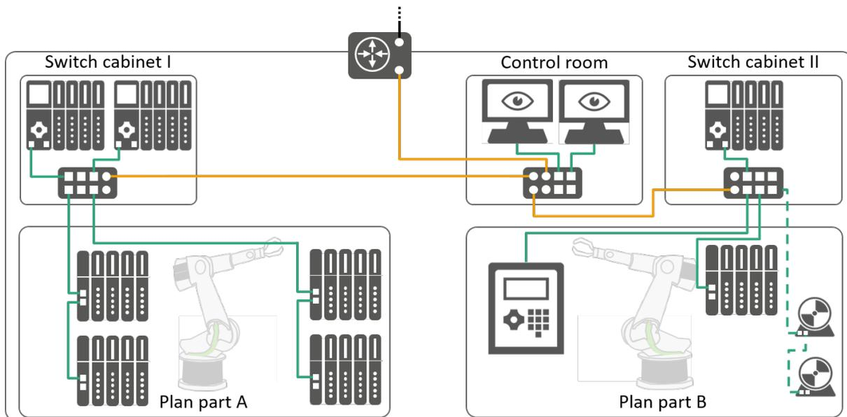
**Figure 6-1: Example of a factory automation**
