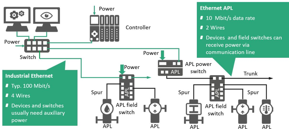
**Figure 5-1: Differences between Fast Ethernet and APL**
