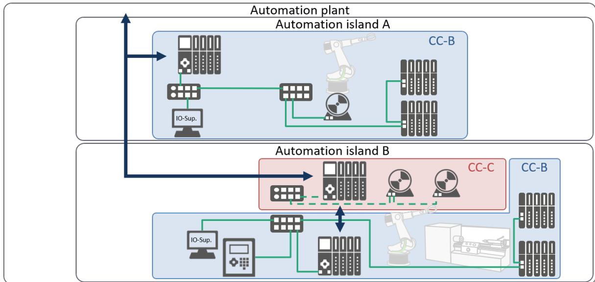
**Figure 3-12: Plant example with additional communication tasks**
