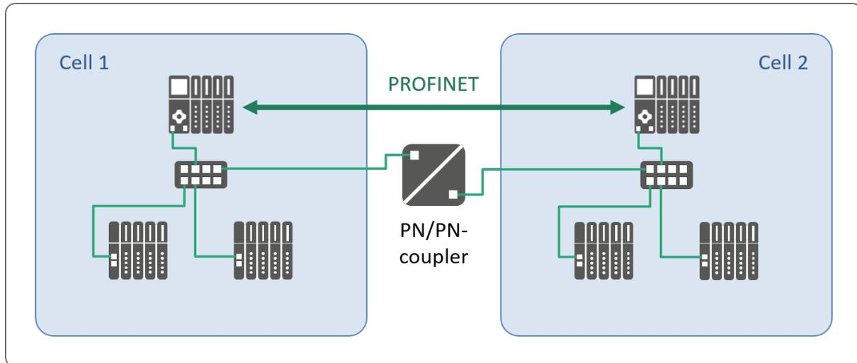
**Figure 3-15: Connection of two functional units with PN/PN coupler**
