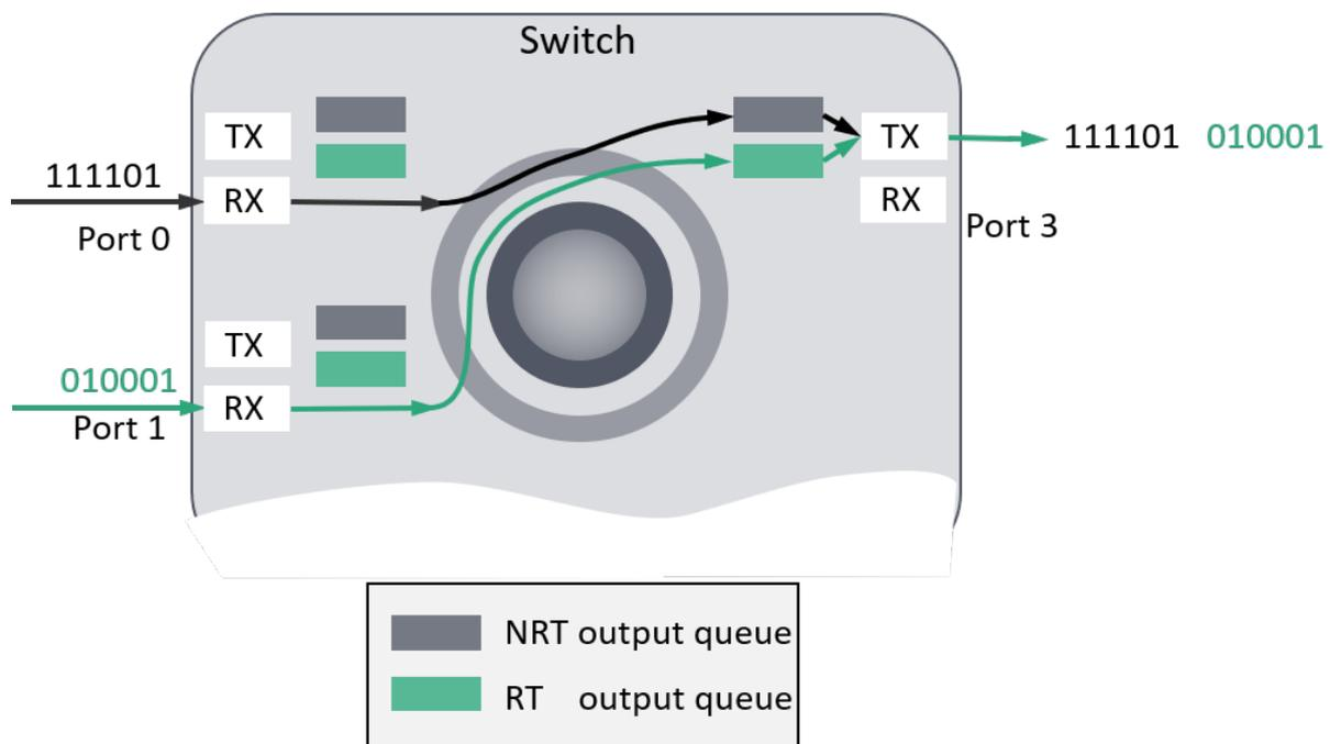
Figure 7-22: Switch principle with queues
