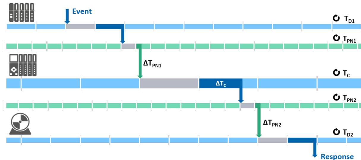
Figure 7-8: Examples of cycles in the processing chain, longest response time
