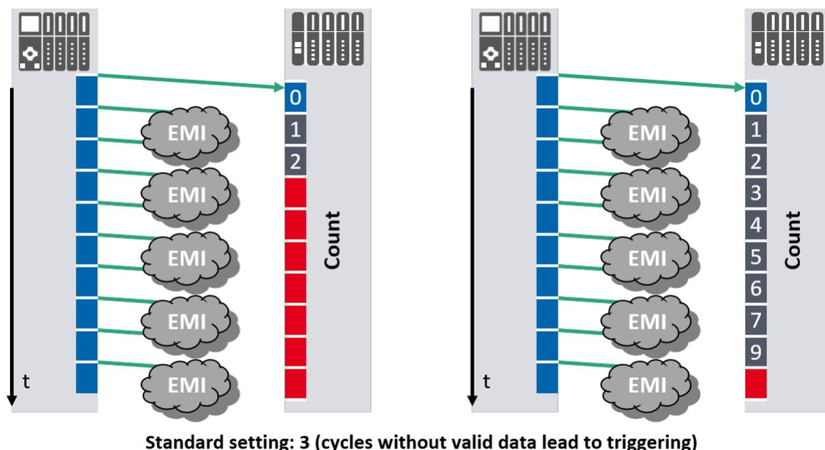
Figure 7-11: Comparison of low (3, left) and high (10, right) threshold
