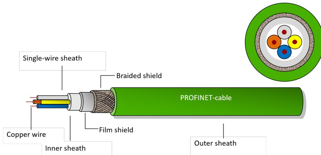
Figure 10-1: PROFINET cable type A
