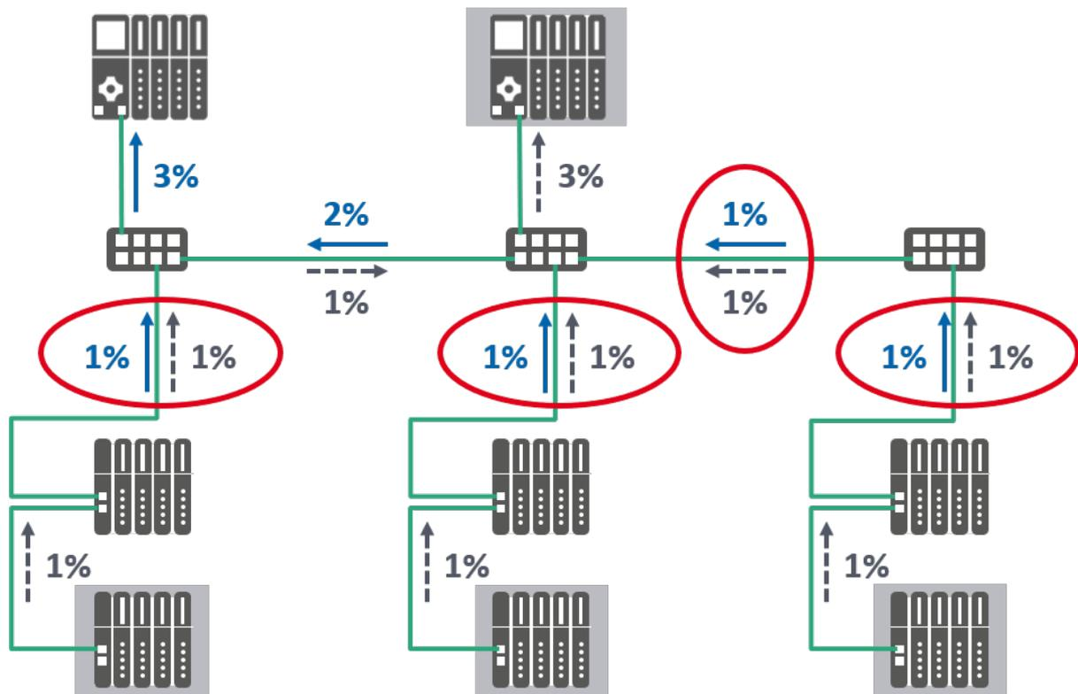
Figure 7-17: Example of network load distribution in a multi-controller application
