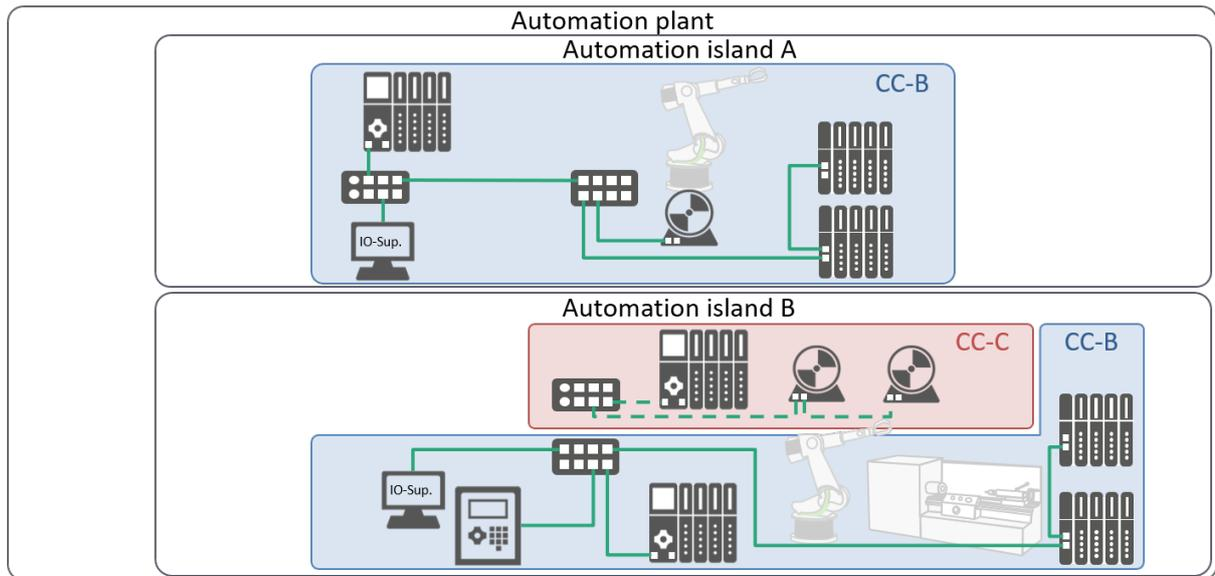
**Figure 3-10: Plant example with interconnected functional units**
