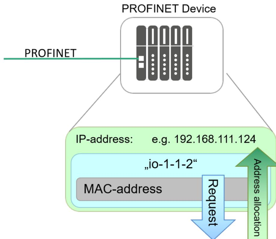
Figure 8-2: PROFINET device (address allocation)
