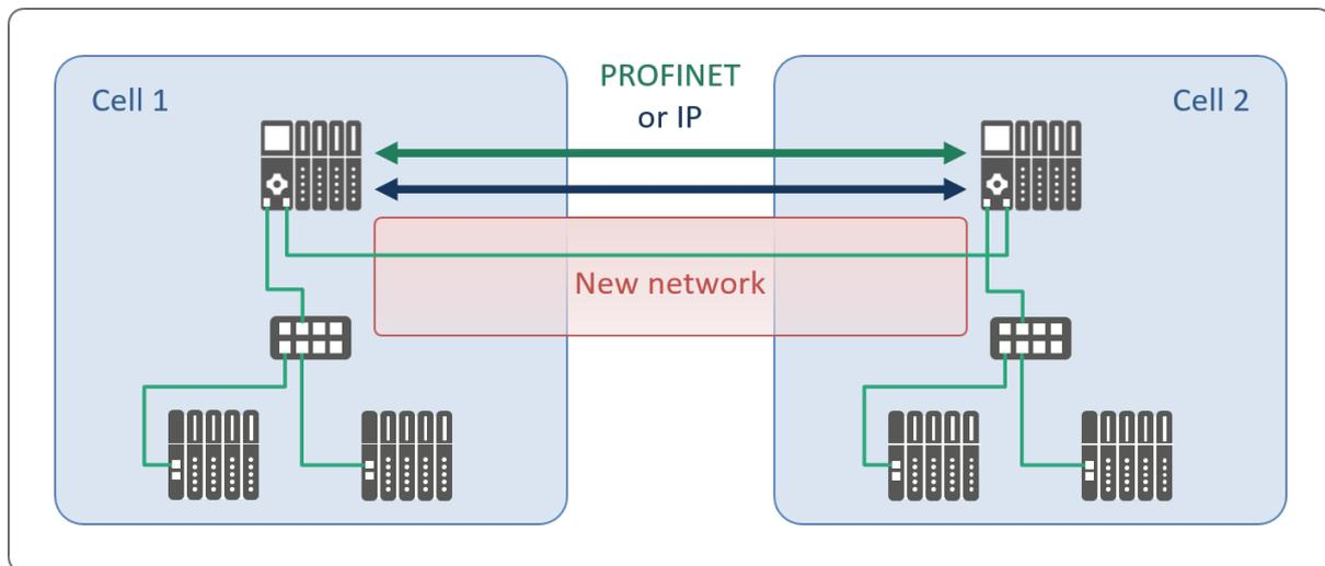
**Figure 3-16: Connection of two controllers via the second Ethernet interface**
