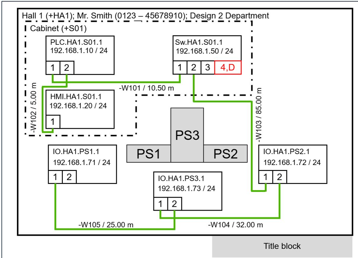
Figure 10-27: Example of PROFINET forwards documentation, physical topology plan
