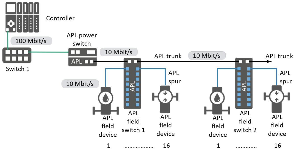
Figure 7-26: System Structure of an APL System with trunk and spur topology
