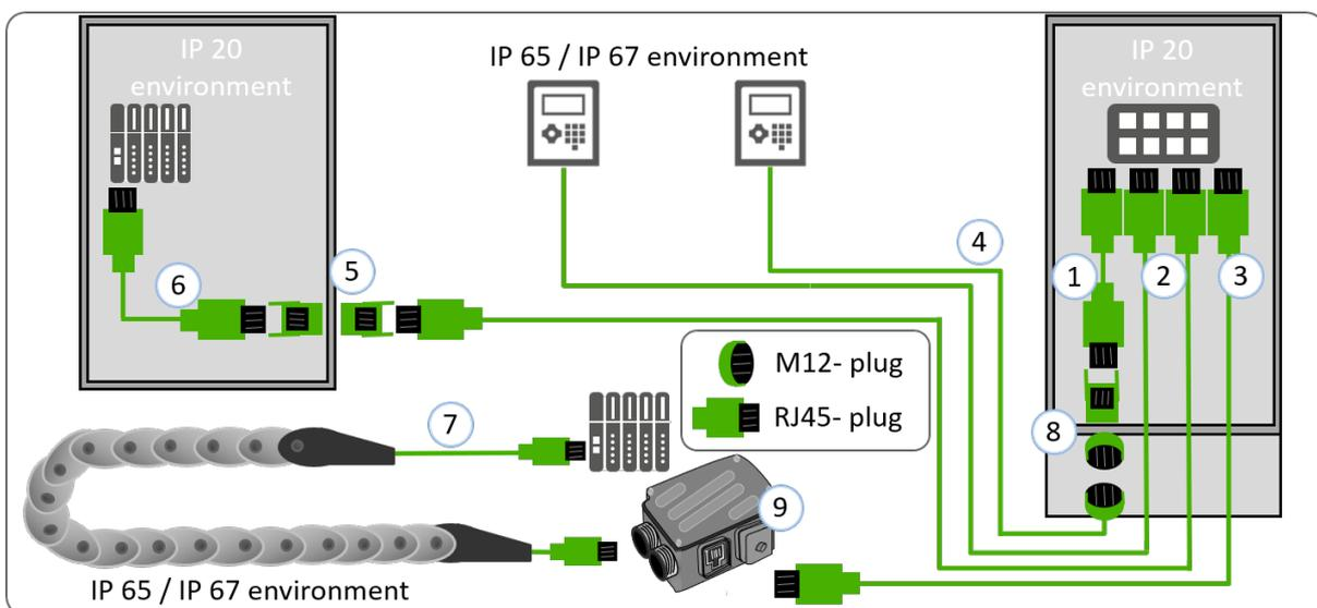
Figure 10-20: Examples of copper-based cabling
