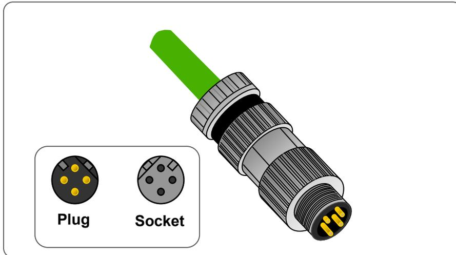
Figure 10-11: Typical D-coded M12 connector
