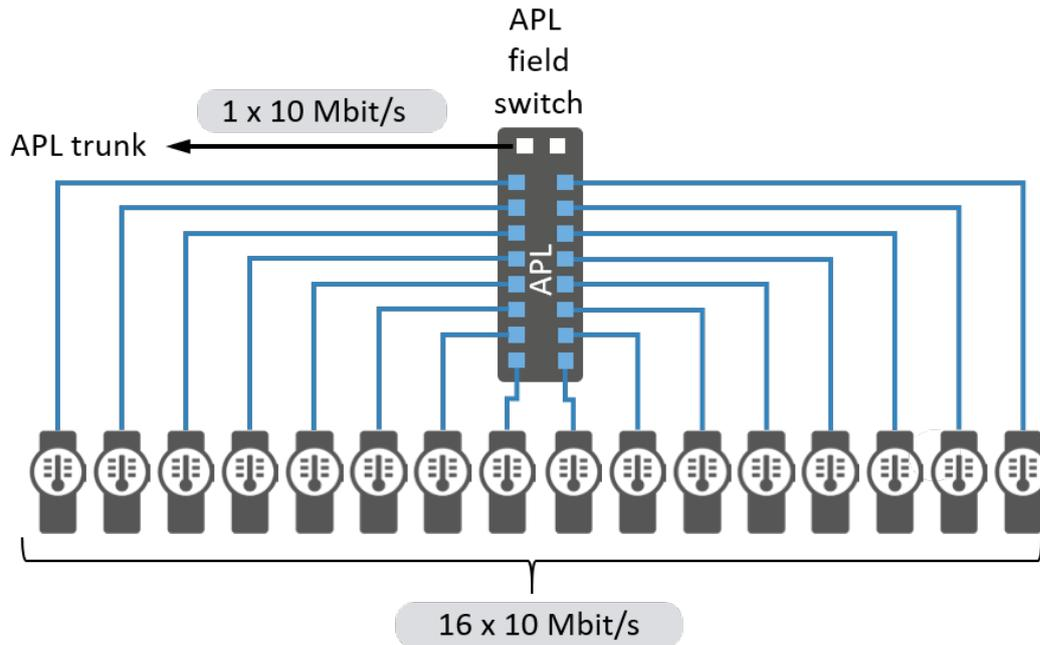
Figure 7-24: Example for input/output unbalance port count wise
