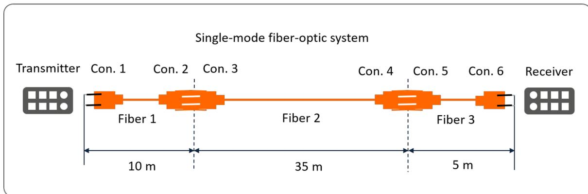
**Figure 10-23: Representation of attenuation balance for POF FO link**
