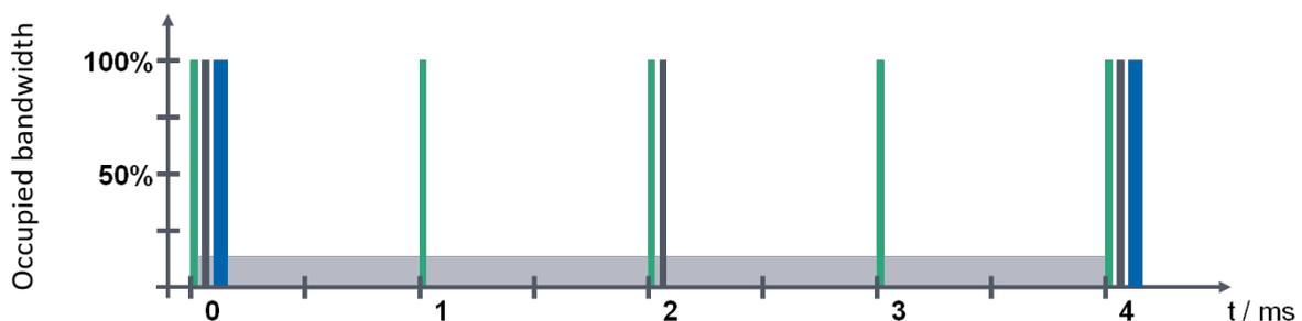
**Figure 7-5: Example of the network load development during a transmission cycle**
