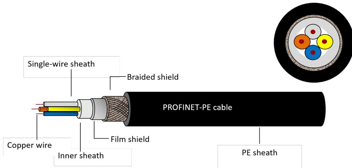
Figure 10-2: PROFINET PE cable
