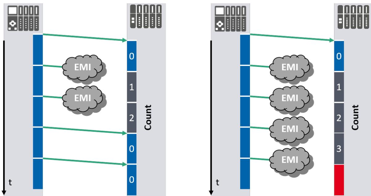
Figure 7-10: Communication problems with error threshold 3
