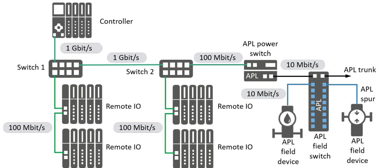
**Figure 7-21: Mixed Link speeds and star topology in a PROFINET system**
