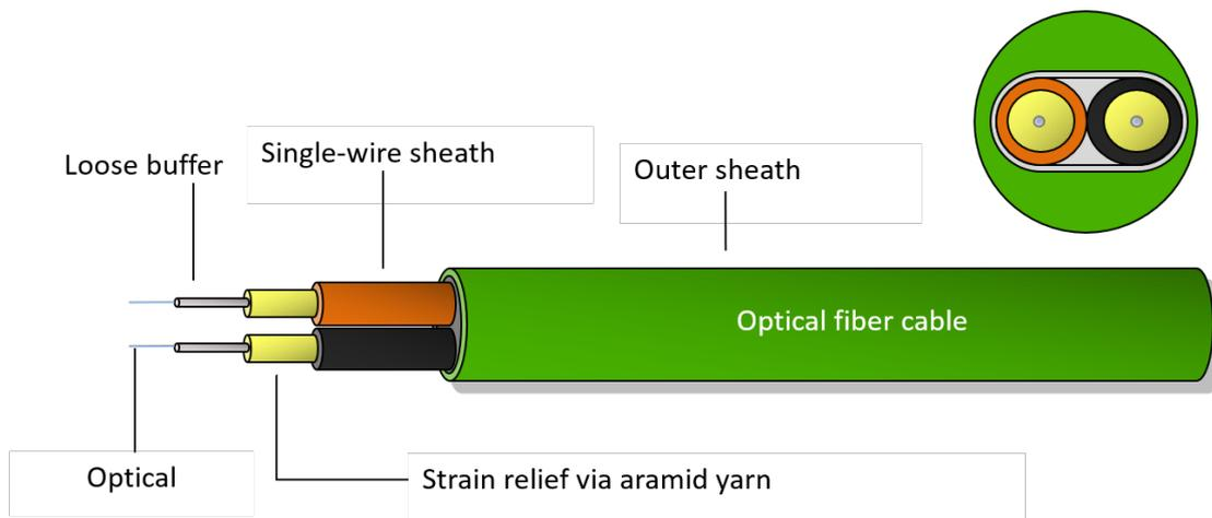
Figure 10-7: PROFINET optical fiber cable
