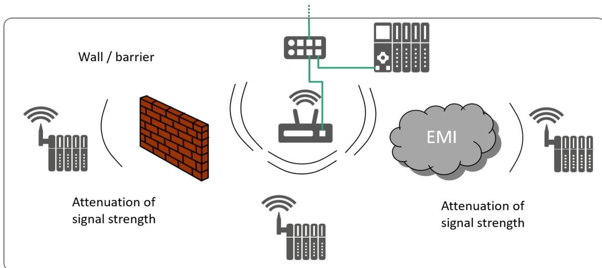
**Figure 4-5: Use of wireless transmission technology**
