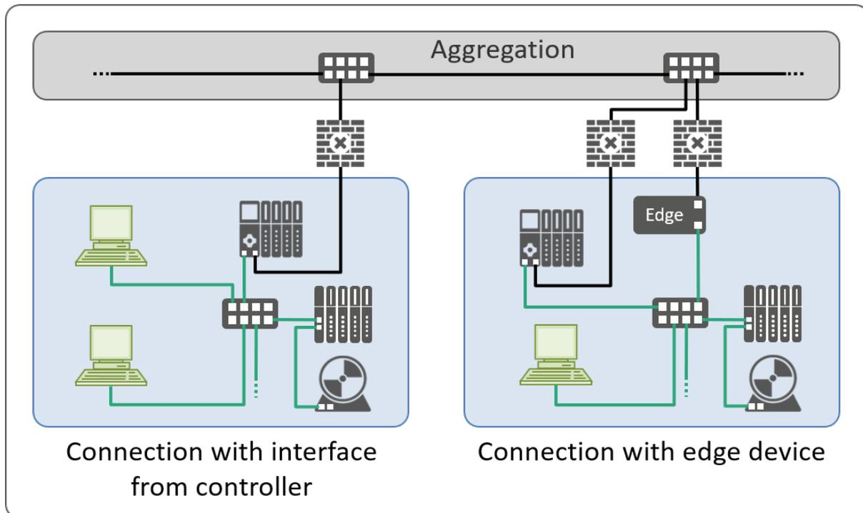
**Figure 3-18: Examples for the connection of separate devices**
