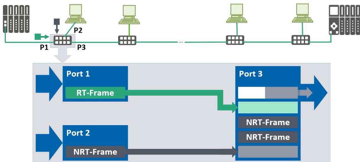
Figure 7-1: Prioritization of real-time communication with PROFINET
