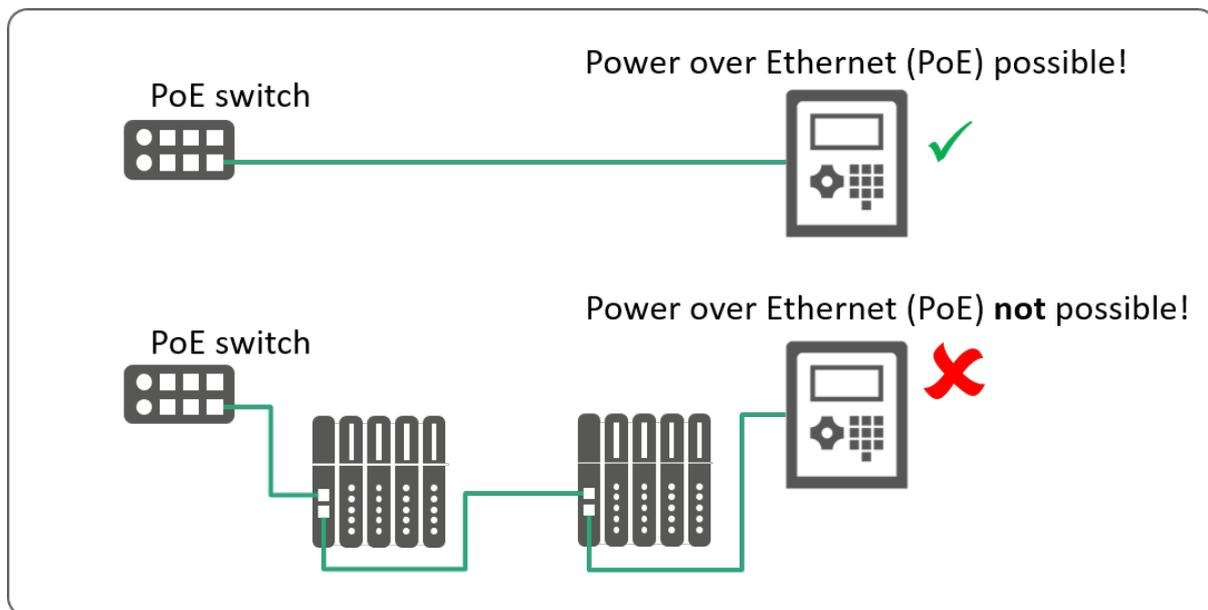
Figure 4-6: Topology limitations with Power over Ethernet
