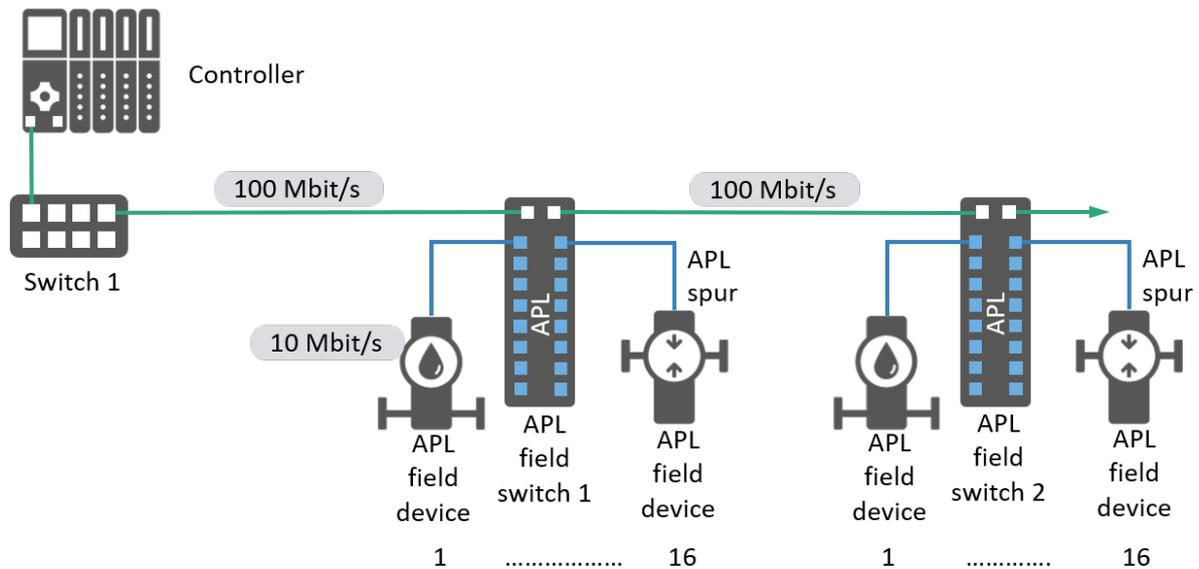
**Figure 7-27: Ethernet-APL system with 100 Mbit/s industrial Ethernet to the field switches**
