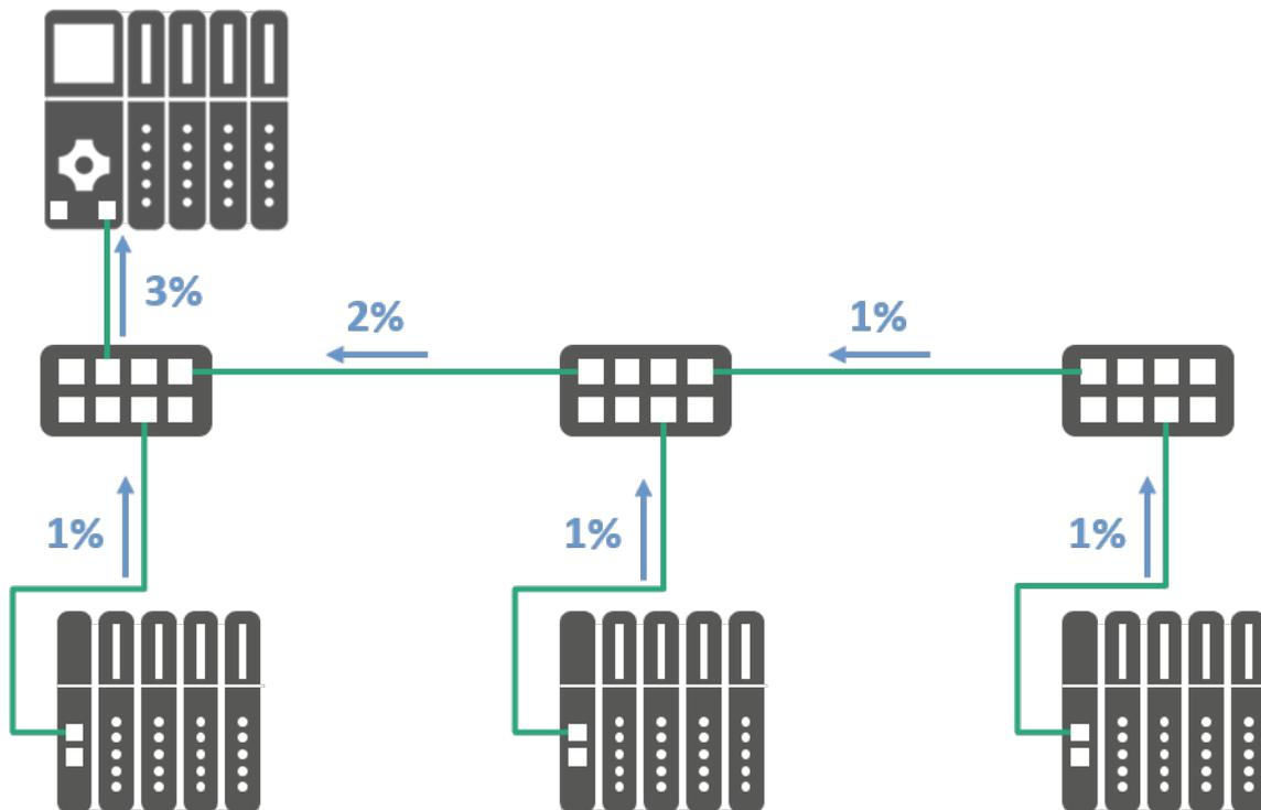
**Figure 7-16: Example of network load distribution in a single controller application**
