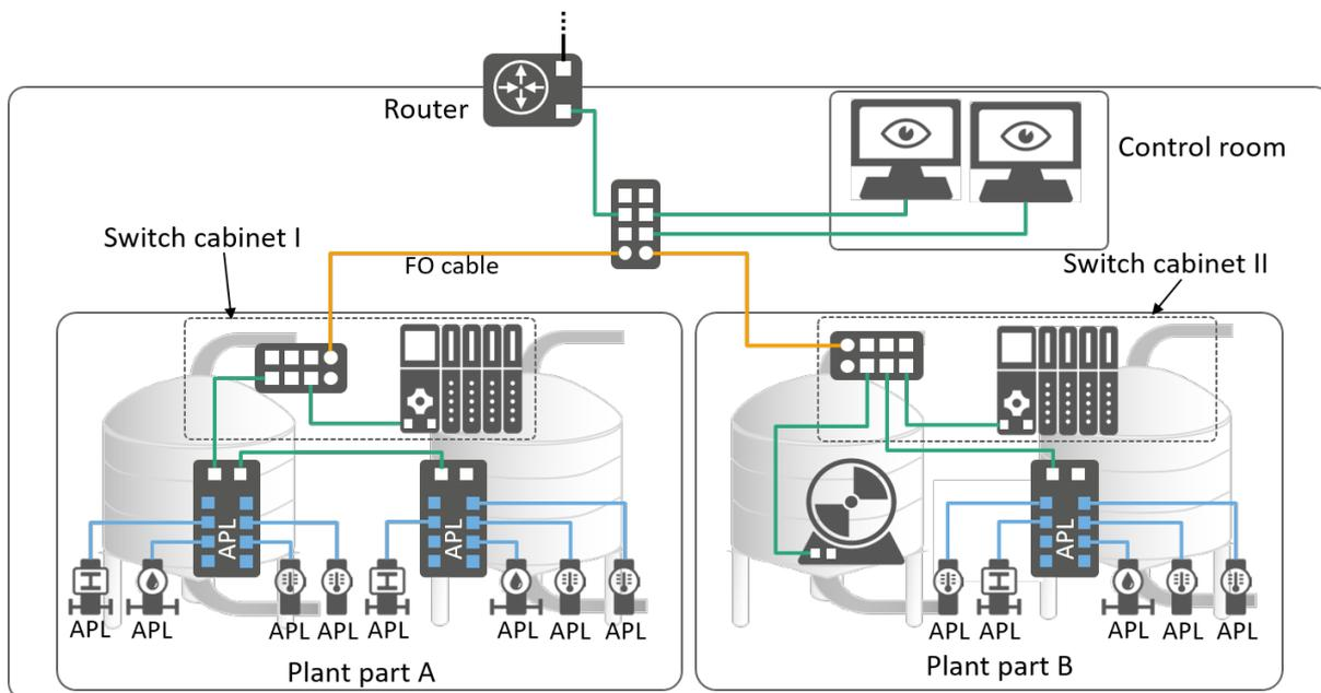
**Figure 6-4: Example Plant Process Automation with Ethernet APL**
