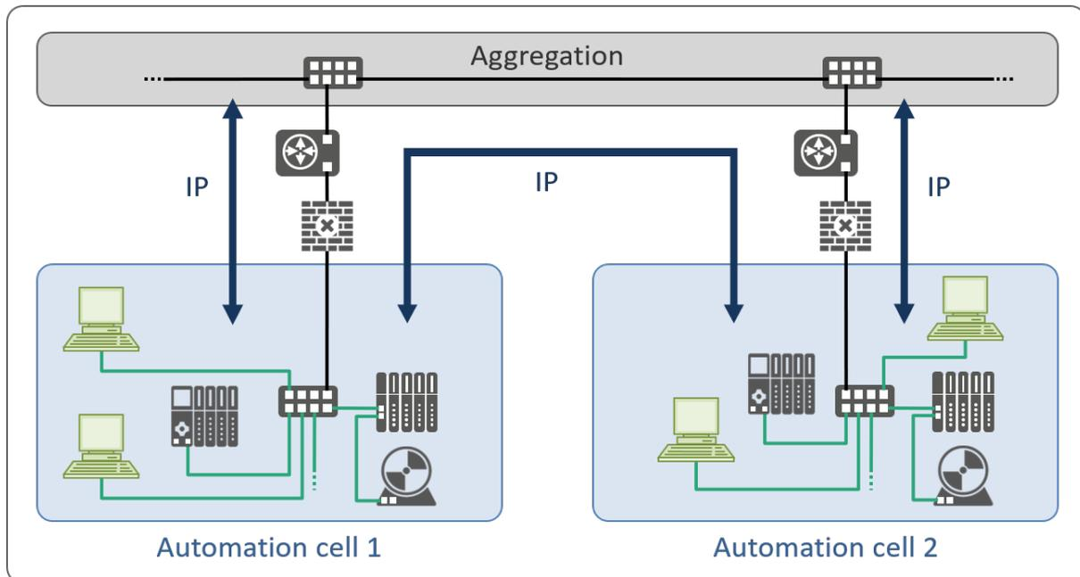
**Figure 3-17: Connection to the aggregation layer with router**
