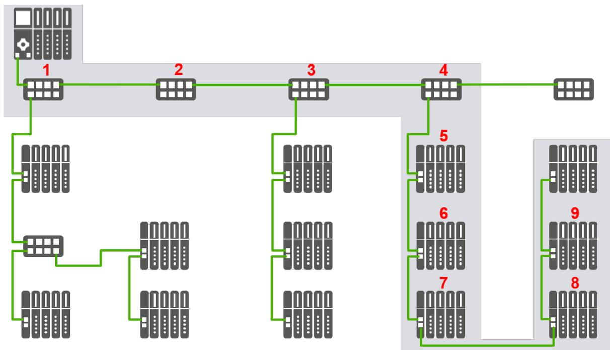
Figure 7-12: Line depth example
