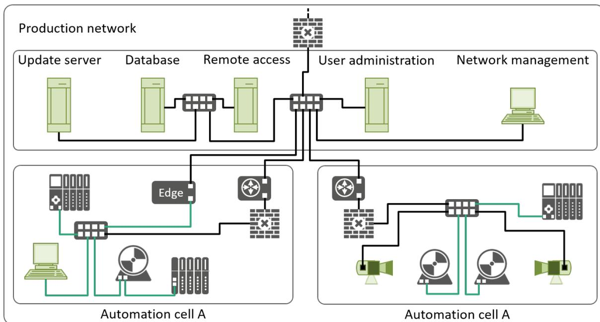
Figure 6-7: Plant example for converged networks
