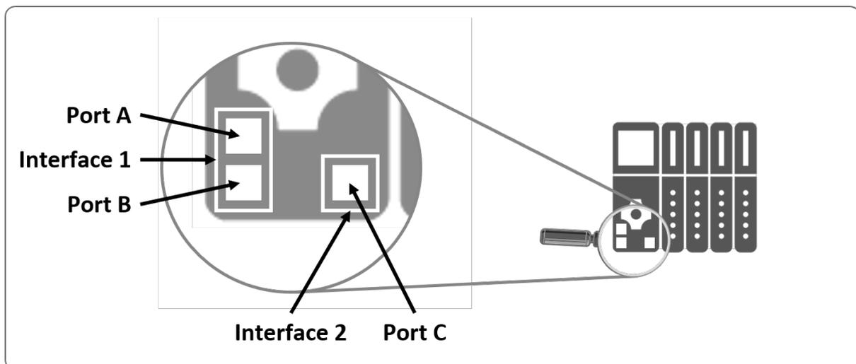
**Figure 3-1: Difference between the terms port and interface**
