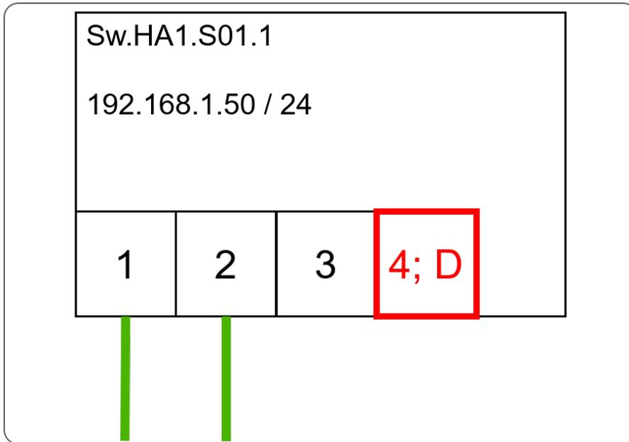
**Figure 10-31: Example of PROFINET forwards documentation, diagnostic port example**
