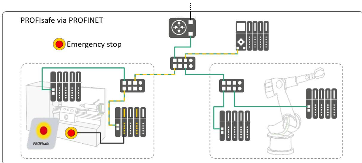
**Figure 2-6: Use of PROFIsafe via PROFINET**
