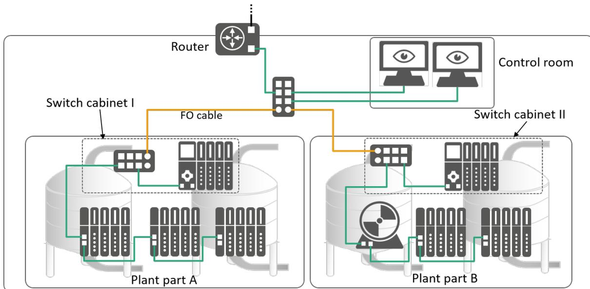
**Figure 6-3: Example plant process automation with remote IO**
