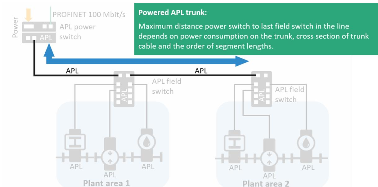
Figure 5-3: Powered APL trunk
