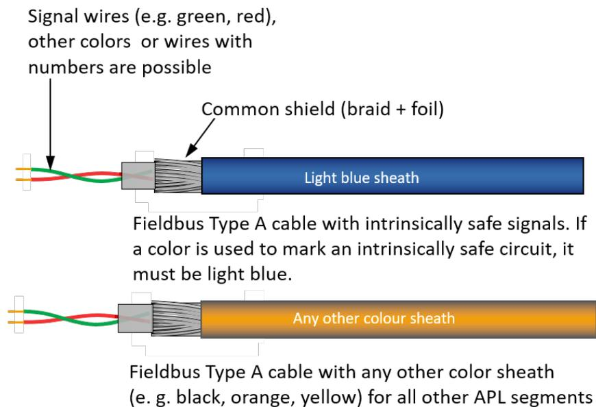
Figure 10-6: Ethernet-APL cable
