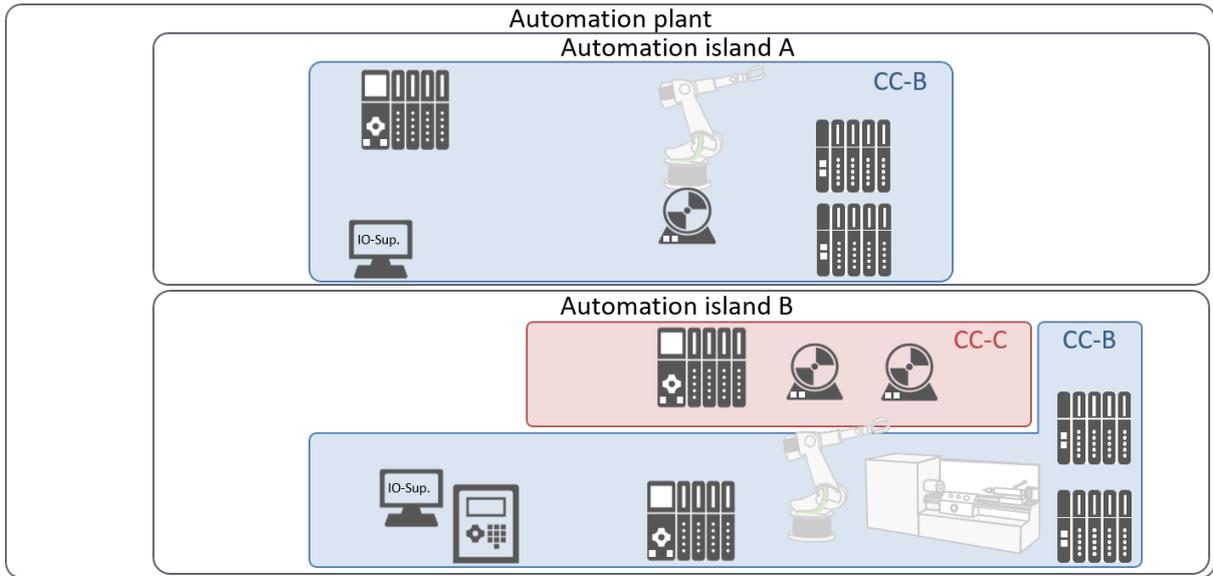
**Figure 2-5: Plant example with conformance classes**
